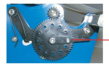
Set the lever pin of the dispensing gear to the desired number of inches of tape feed. This will permit only the selected length of tape to be dispensed on each pull.
