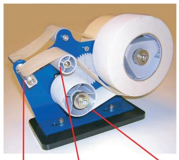
Feed tape backing onto the take-up roller from its underside.
