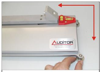
Level the Auditor MSM as accurately as possible using the built in bubble level. Leveling the instrument is done by dialing the leveling feet.
