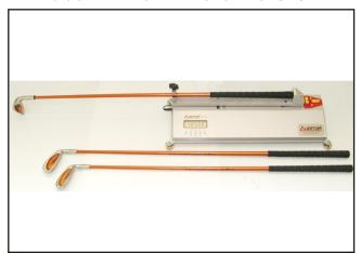
Mount the first club on the beam and take an MOI reading. Press **ZERO** to clear the display and remove the club. Mount the 2nd club on the instrument and take a measurement. The reading is the MOI difference.
