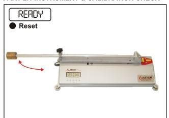
The Calibration stick will oscillate gently for few seconds before the measured MOI value is displayed. Note the value mentally and press the reset button again to take a second and a third reading.
