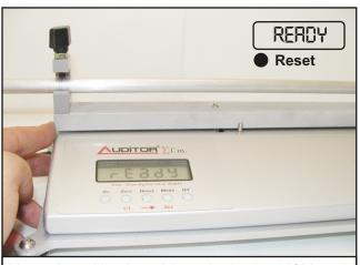
Mount the calibration stick on the Auditor MSM, and gently pull the beam until it contacts the side stop. Release the beam and press the reset button
