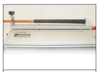
When placing a club on the beam it is not necessary to tsecure the club with the thumb screw, as long as the club points toe towards the ground and does not wobble during an oscillation cycle.
