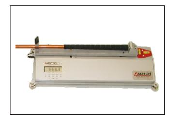
The MOI measurement is in Kg.Cm^2 by default. To convert to Lb.In^2 press MODE to toggle between the two sets of units. Slug.Ft^2 is not an available option on this instrument.
